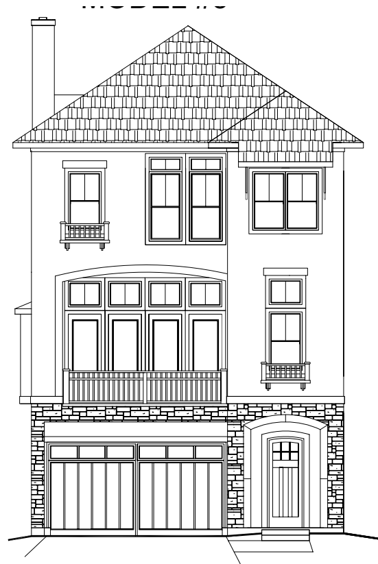
STUCCO / STONE / COMPOSITION ROOF
