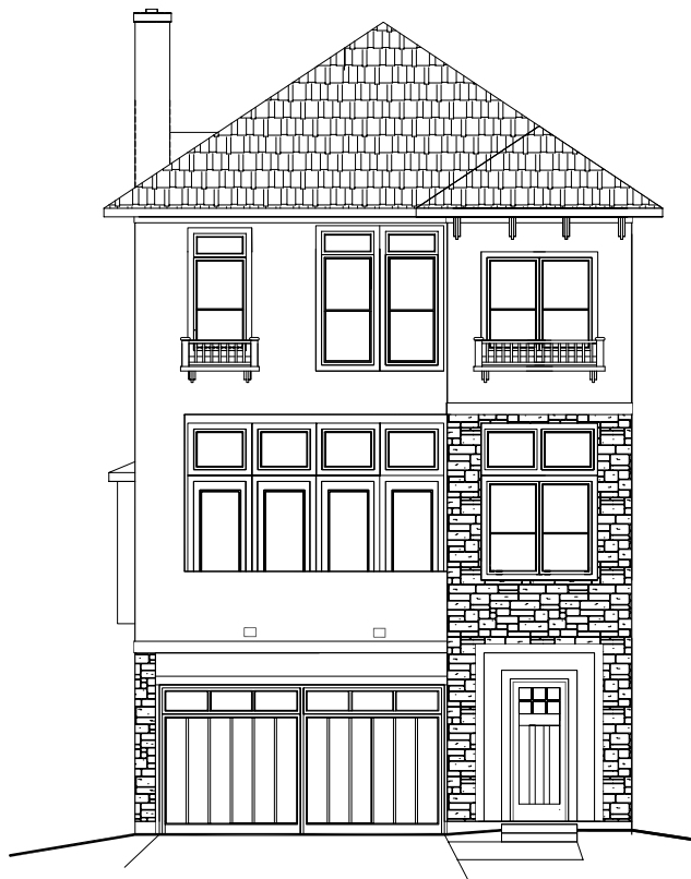
STUCCO / STONE / COMPOSITION ROOF
